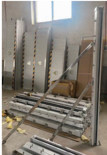
2 or 3 pcs of support braces can be applied on high center post.
